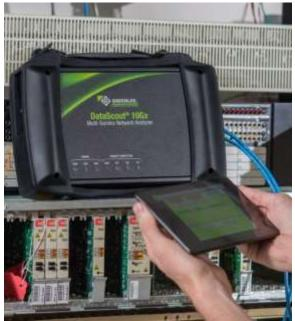
enables technicians to work independently of their test equipment and enhances safety by allowing technicians to step away from noisy or cramped work locations and work from a safer area."
